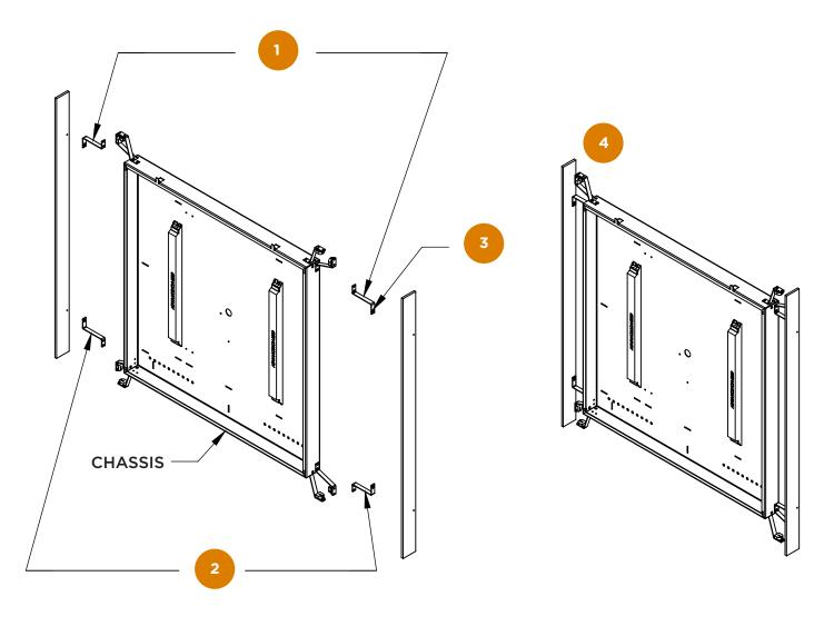
1 Attach top diffuser brackets to Chassis with (2) included #8 X 3/16" Long Pan head screws align back of brackets to back of Chassis
